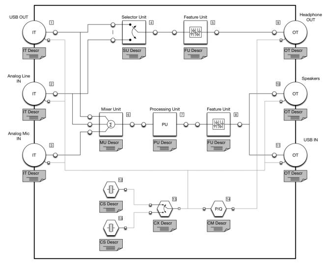
Figure 3-3: Inside the Audio Function
